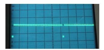
At the Fastest position and using the trimpot P1 to trim for about 99% pulse width. If you over trim then the 556 will 'trip-over' itself and the motor speed will drop. Here is what you see when you just over trim the trimpot from the above photo.
