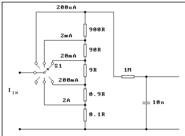
Figure 4 Multirange Current Meter.
