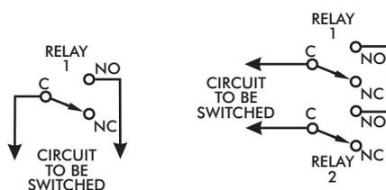
**Fig.3a (left): conventional device control with one relay. Adding a second relay in series (fig 3b, right) increases security against the casual button pusher. Both buttons must be pressed at the same time for the device to actuate.**
