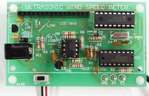
underneath the PCB. Pads labelled 12 and 13 under the PIC firmware are for switches S2 and S3 resp. (Remember pin 12 for S2; pin 13 for S3.) Add about 6" of wire from these pads and the two GND pads provided. S2 and S3 are needed for testing and minor calibration later. Label the two switches.
