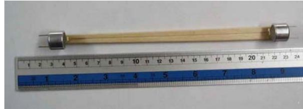
Make sure they face each other squarely. When set we joined the two earth pins with green wire. Connect the assembly to the PCB using three wires: GND, X4 and X3. You can use the pins provided or solder direct to the pads. Note each ultrasonic transducer is treated the same. No track needs to be kept of which is the Tx and which is the Rx. See the EPE article for more details on this.
