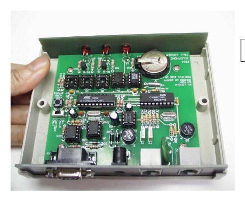
One out of the 4 memory chips is inserted.
