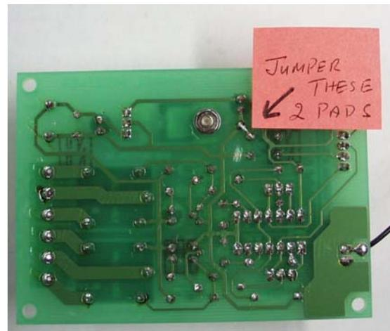
Connect the other side of the tact switch to ground as shown. Use an offcut from resistor leg. See it at <http://www.kitsrus.com/jpg/k157jump.jpg>
