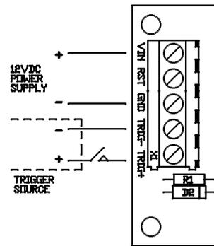
Fig 3. Electrically isolated triggering
